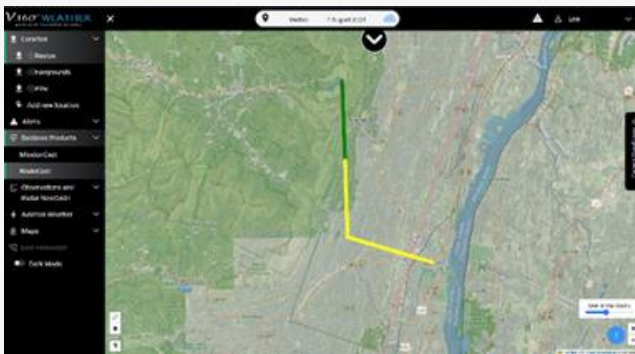
Figure 4 and 5: Side by side comparison of wind thresholds (V360 Weather, RouteCAST Decision Tool). By changing the flight path, the drone can reach its destination in a shorter amount of time and with more battery life.
