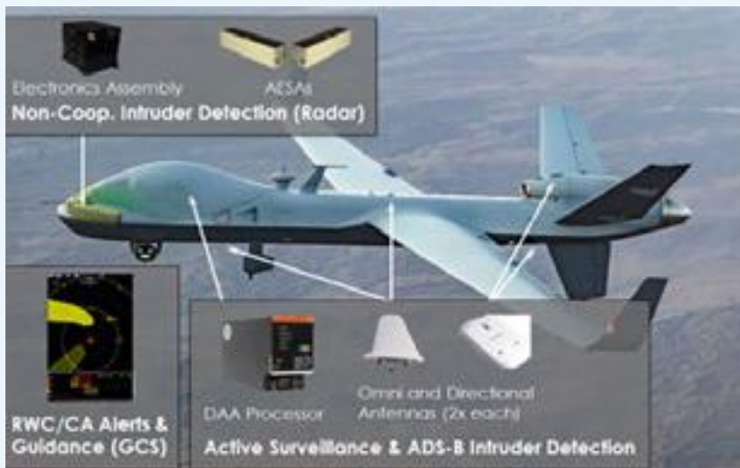
Typical DAA Installation
